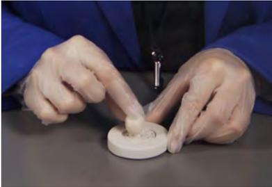
**1** First press the Ceralun into the 3D silicone mold to form the required shape.
