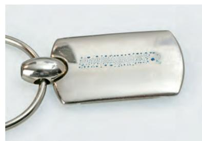
**3** If the ink disappears or forms bubbles, the surface is not suitable for applying Ceralun. In this case, the pre-treatment cleaning methods should be checked.
