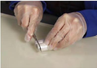
**1** Cut off resin and hardener with a knife.
