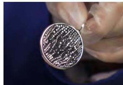
**3** After removing the pattern from the clay, the crystals can be set.
