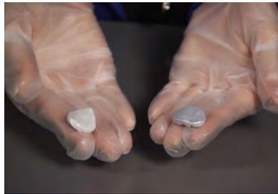
**2** Weigh the two components. The mixing ratio for Ceralun is 1 : 1 by weight.
