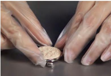
**4** After taking the mold out of the freezer, the Ceralun can be removed from it and gently pressed into place on the chosen object.
