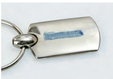
**2** If the ink remains visible for 2 seconds, the surface is suitable for working with Ceralun.
