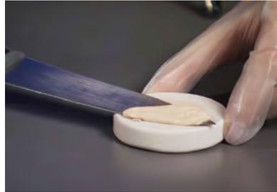
**2** Any overlapping material can be trimmed off with a knife.
