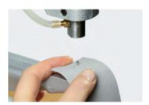
**6** Put the carrier material with the pre-punched hole over the lower part.
