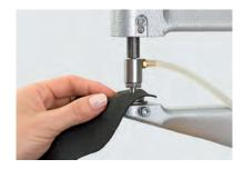
2 Position the carrier material and apply. Regulate the offset/pressure using the adjustable stop.
