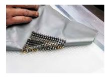
18 Press with a cutting press and apply the 3D Studs all at once. Keep the vacuum system on until the end of the application.
