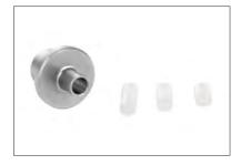
3 Choose the matching insert for applying a 3D Stud of another size and push it into the lower die. Make sure the cavity of the insert is located at the upper side of the tool.
