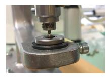
Before starting the application make sure that upper and lower die are positioned in the center. Pre-punching the fabric and positioning it properly on top of the lower die guarantees the correct functionality of the finished product.
