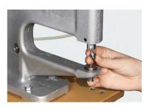
1 Replace the upper and lower die in order to apply the Snap Fastener closure.
