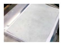
**16** Remove the middle metal plate and lay the fabric in the mold.
