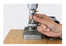
1 Place the 3D Stud in the lower die, with the crystal side pointing downwards.
