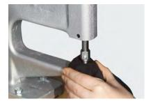
3 Apply the product on the carrier material. Adjust the offset/pressure using the adjustable stop.
