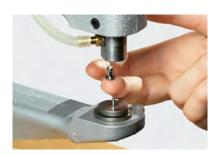
5 Place the upper part in the upper die (crystal pointing upwards).
