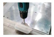
1 Before starting production with a new motif, the vacuum suction has to be installed in the mold. Open the cover's plates by unscrewing the screws with a drill.
