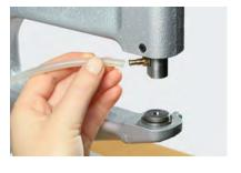
${\bf 3} \quad \hbox{Connect the vacuum pump and turn it on}.$
