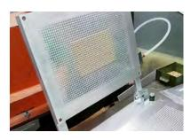
15 Switch on the vacuum system, close the cover and then open it again. The Back Parts are now inside the cover.
