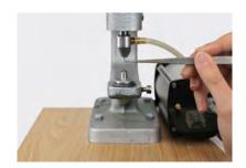
2 Attach the vacuum pump to the upper die and turn the vacuum pump on. The Back Part can now easily be positioned into the upper die with the arrow pointing downwards.
