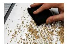
13 Empty the Back Parts into the black frame. Use the sponge to wipe them into the mask's cavities (arrows pointing downwards).
