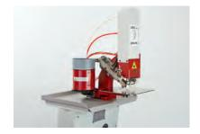
Some Swarovski products can be applied using a semi- or fully-automatic attaching machine (e.g. Rose Pins). In this process, the feed on the machine must be adjusted to the product being processed.
