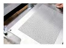
**9** Put the middle metal plate back into the mold.
