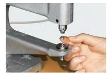
2 Place the ball part in the upper die (will be kept in position by vacuum) and the counterpart in the lower die.
