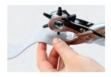
Pre-punch the carrier material on the designated position for the Crystal Stud.
