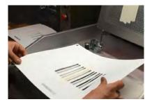
5 Remove the middle metal plate and put the first PVC mask onto the lower part of the mold.
