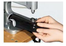
3 Apply the product on the carrier material. Adjust the offset/pressure using the adjustable stop. Check the functionality of the Snap Fastener after the application.
