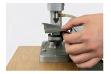
3 Turn the fabric with linear grid around and put all parts into the fly press on top of the lower die. Activate the vacuum pump and fit the Back Part into the upper die. Apply the 3D Stud by closing the handle of the fly press.
