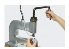
**7** Apply the Crystal Stud by closing the handle.
