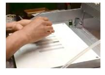
6 Insert the first pins into the mask's cavities (colored part upwards) as height compensation for the corresponding 3D Studs. Use one mask and pin color for each 3D Stud size and repeat the setting step for all masks.
