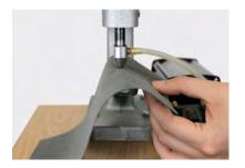
3 Position the carrier material with the right side pointing downwards. Apply the 3D Stud by carefully closing the handle of the fly press.
