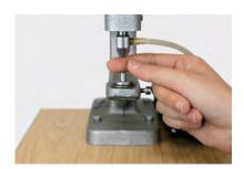
1 Set a 3D Stud (crystal pointing downwards) in the lower die with insert.
