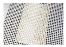
14 Remove the residual Back Parts, the black frame, and the masks. Make sure the middle metal plate stays in the mold.
