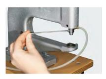
Place the vacuum adapter and the tools in the fly press. Make sure that they are fixed and connect the vacuum adapter to vacuum pump.
