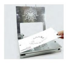
1 Put the first PVC mask onto the lower part of the mold.
