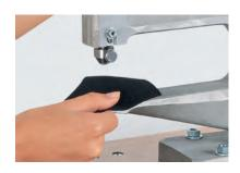
**3** Apply the product to the textile in the previously marked position. Regulate the offset/pressure using the adjustable stop.
