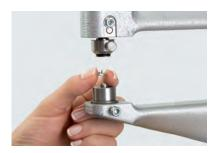
1 Place the pronged ring in the lower die, with the prongs pointing upwards.
