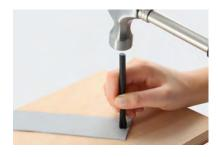
**9** Create the buttonhole with a buttonhole punching tool (art. 9040/122).
