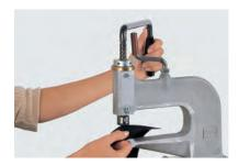
3 Carry out the application in the desired position. Regulate the offset/pressure using the adjustable stop.
