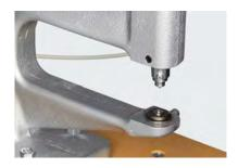
2 Place the decorative part in the upper die and the spring socket in the lower die. The vacuum will keep the decorative part in upper position during application.
