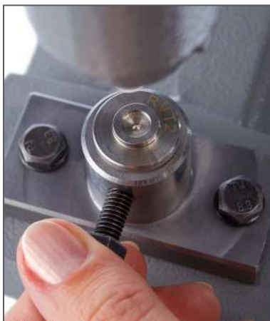
4. Tighten the lower die.
