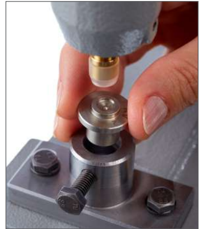
3. Placement of the lower die.
