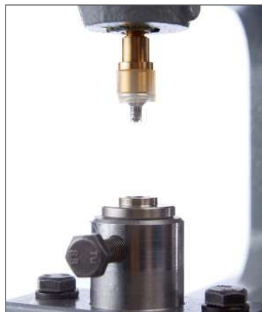
5. Attach the rivet to the upper die.
