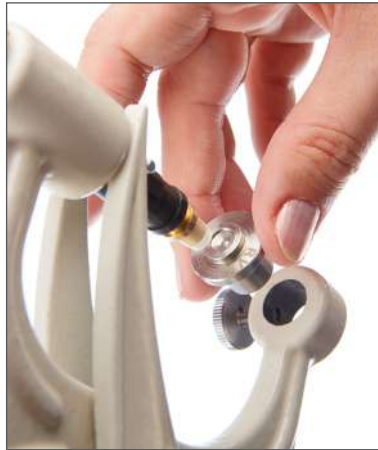
2. Placement of the lower die.
