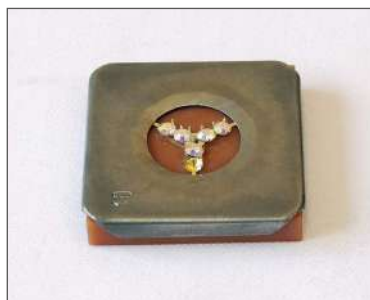
Device for manual setting of rhinestone balls
