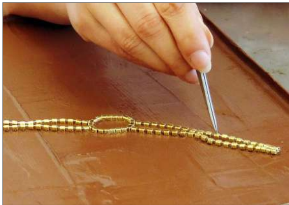
7 Check if the parts in the impression are placed according to the sample.
