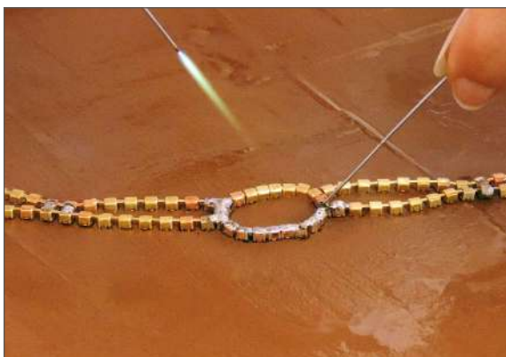
11 Repeat the soldering in chosen parts of the jewellery article.
