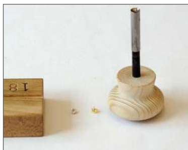
Setting and closing tool for individual cups
