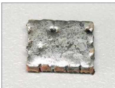
Too much solder (the solder flows over the cups)
